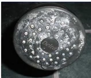
This photo shows the same showerhead on November 7<sup>th</sup>, 2009, just over five weeks after installation of the Aqua-Rex. The original scale remains on the showerhead but no additional scale has been deposited.
