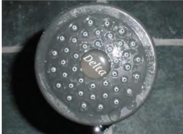
This photo shows what happened after the showerhead was wiped with the thumb. The scale is now soft and can be wiped off without using any chemical cleaner, leaving the showerhead almost completely clear. The Aqua-Rex unit has softened the scale and reduced its adhesion to the showerhead surface. It has also stopped new scale from forming and the tiles were also clean.
