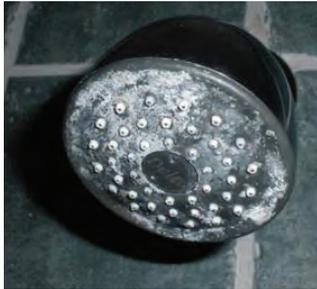
On the left is a photo of the showerhead in the left hand cubicle of the women's locker room on October 1<sup>st</sup>, 2009. The scale on the showerhead was hard and encrusted and could only be removed by using an acid cleaner.
